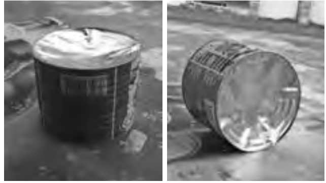
The bottom of the measuring tin has been knocked in.
